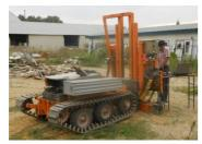
Seismic Cone Penetration
