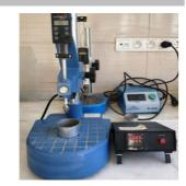
Fall Cone Test Device
