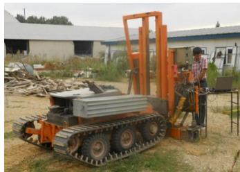
Seismic Cone Penetration
