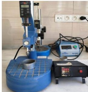
Fall Cone Test Device
